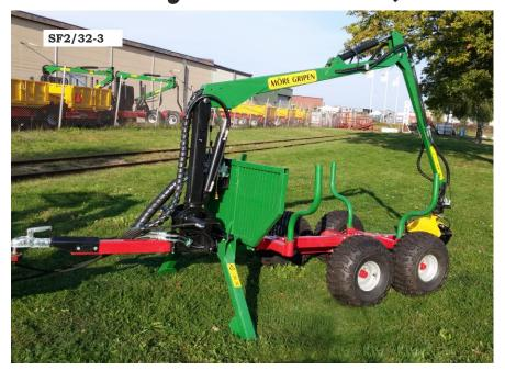
Forestry trailer with centre frame, adjustable bogies, removable pivoted supports, easy-to-use valve block, retractable support legs, coupling for tow ball
