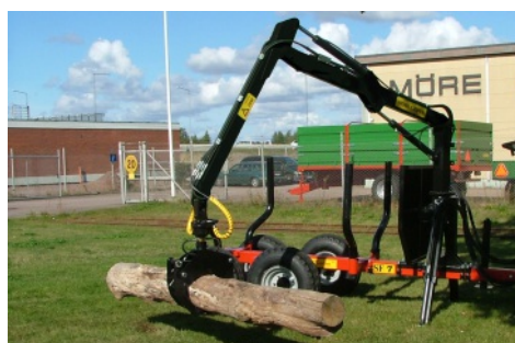
Forestry trailer 7 tonnes, centre frame, bogie wheels, hydraulic support legs, pivoted supports, tow ring for tractor
