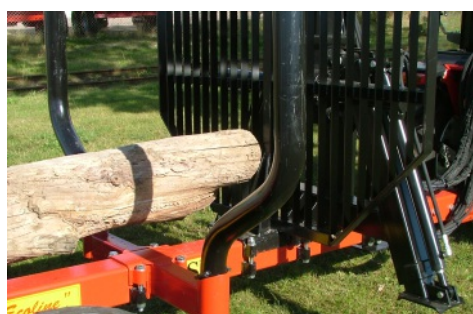
Forestry trailer 7 tonnes, centre frame, bogie wheels, hydraulic support legs, pivoted supports, tow ring for tractor
