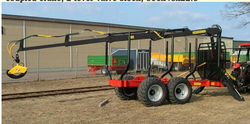
Forestry trailer 14 tonnes, designed for large cranes, double frame, articulated steering, long bunk area, bogie, quick coupled crane, 2-lever valve block, 500x45x22.5
